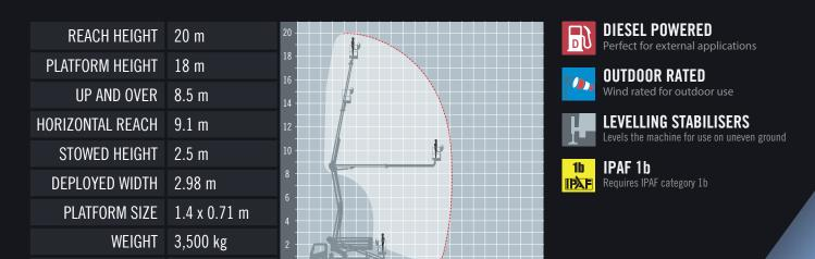
The Isoli PNT 205N truck mounted access platform is perfect for multi-site roadside work or access in tight spaces. Its quick and easy to set up and incorporates a dual articulating boom with a telescopic upper boom that provides great reach from a compact 3,500 kg chassis. At just 3.5 tonne this self drive vehicle can be driven on a standard car licence.
